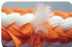
Two or three strands have been cut in this rope
