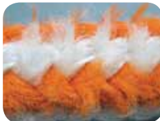
A severely abraded rope
