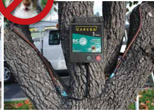
The charger's two D-Cell batteries will power the system for about 60 days.
