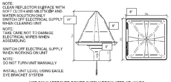
USE ONLY APPROVED POWER SUPPLY REGULATED AT 12V DC NOTE: EAGLE EYE™ ONLY TO ROTATE ANTI CLOCKWISE WHEN VIEWED FROM ABOVE
