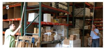
With one person on each end, carefully lift the extension poles and walk the net assembly to the target area. Once in the correct area, lift the extension pole and attach the tip to a rafter or other structure. Or use the hooks provided in the kit if the magnetic adapter is not appropriate. FOR SAFETY: D0 NOT LEAVE THE HANGING NET ASSEMBLY UNATTENDED.
