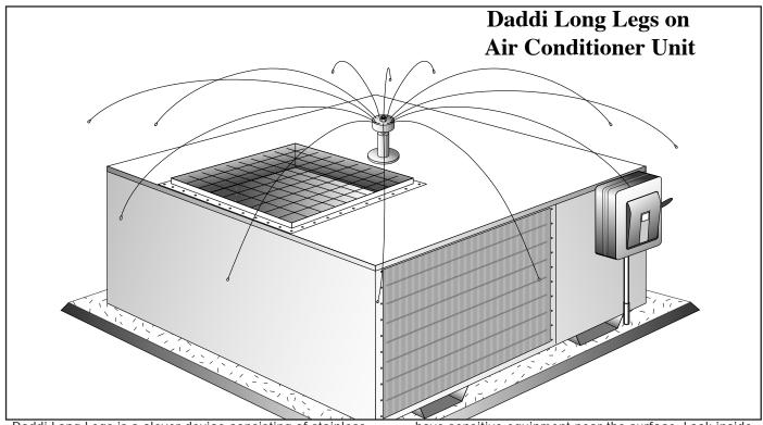
Daddi Long Legs is a clever device consisting of stainless steel rods which extend from a Delrin base. It rotates in the breeze interfering with the birds ability to land. Because Daddi Long Legs is a low-visibility product, many cities and shopping malls have made this their product of choice for their street lights and air conditioning units.
